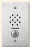
LE-SS-1G Audio Door Station • Stainless steel • Flush mount • Fits 1-gang box (internal door station dimensions are 2-15/16" H x 1-15/16" W x 1-13/16" D)
